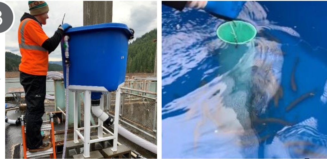
Pull center standpipe Enter Floating Screen Structure (FSS)
